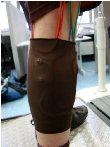
(d) An elastic sleeve helps secure the electrodes to the skin allowing a good measurement of EMG to be taken.
