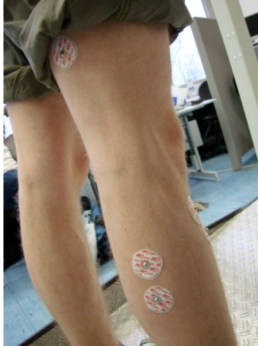
(b) Electrodes connected to the leg muscles to measure EMG.
