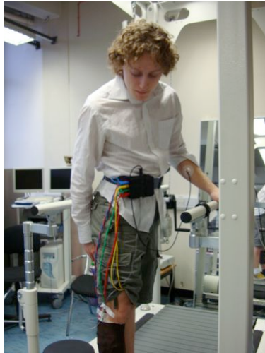
(b) The enclosure containing all the circuitry is securely attached around the subject's waist, wires are connected to the electrodes on the leg muscles and to a ground connection on the left arm.
