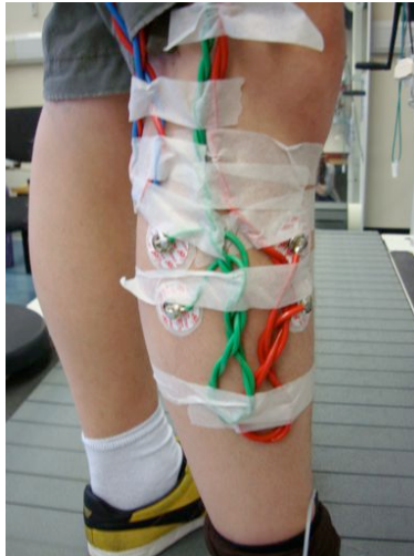
(e) Medical tape was used along with the elastic sleeve to reduce the amount of D.C drift in the EMG measurements.
